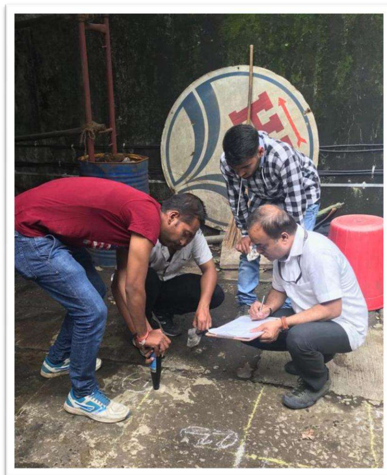
Photo 2. Rebound Hammer Test
