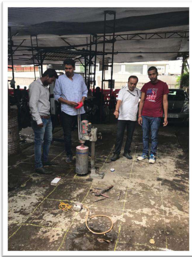
Photo 1 Core Testing Arrangement
